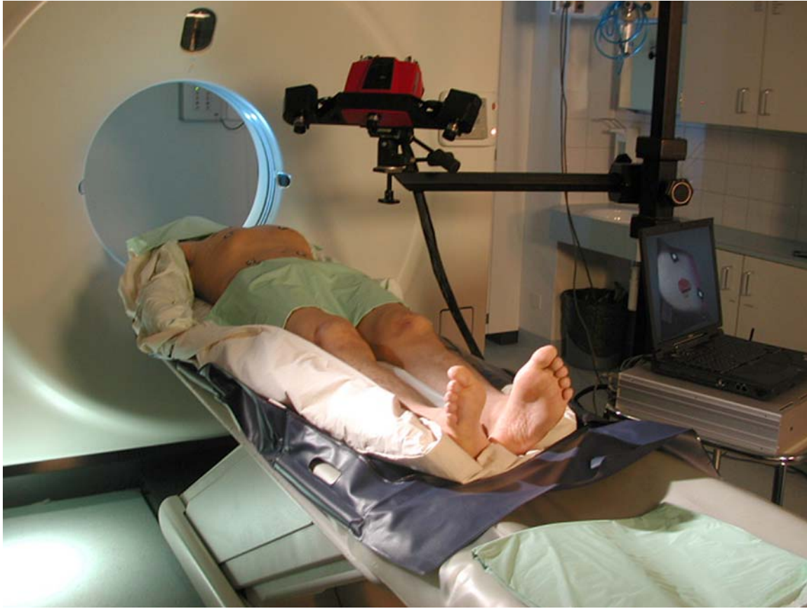
FIG. 20—Modern virtual autopsy table: Set-up of the combined tools of 3D surface and radiology scanner.
