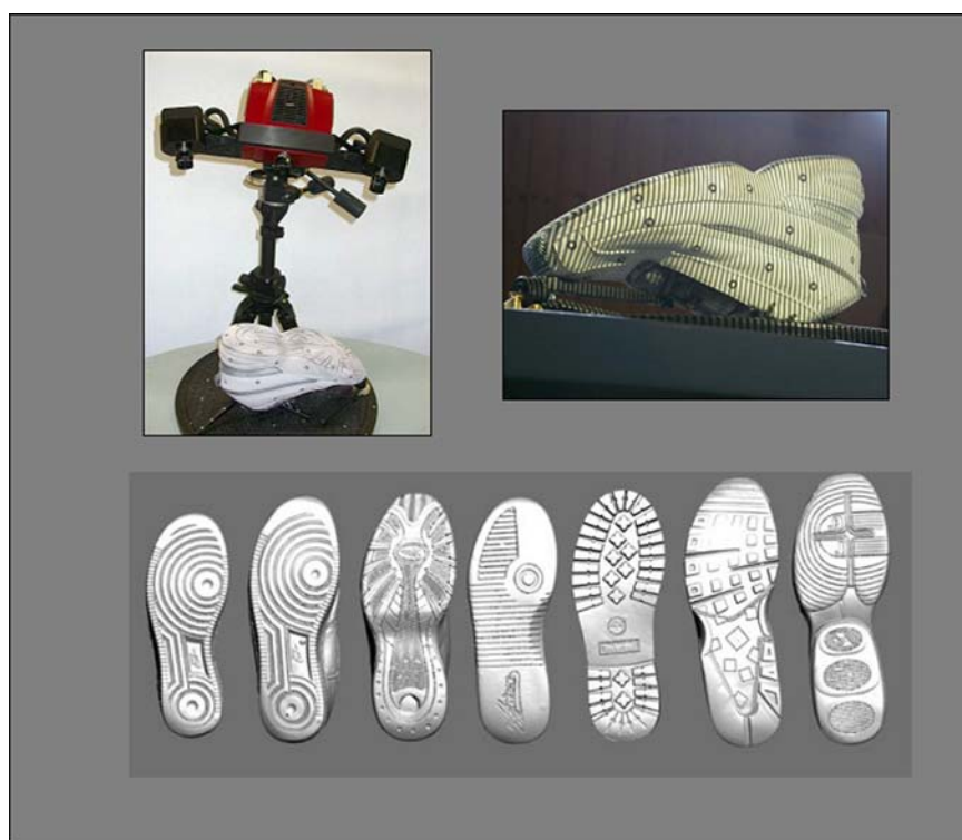
FIG. 2—Case 1: Scanning of the suspected injury causing instruments (upper left) or the soles of different shoes using the optical 3D scanner. The upper right picture shows the fringe projections on the shoe during the scanning process. The lower row of pictures demonstrates the results of the 3D scanning: the 3D individual data models of the shoe soles of the suspected perpetrators.
