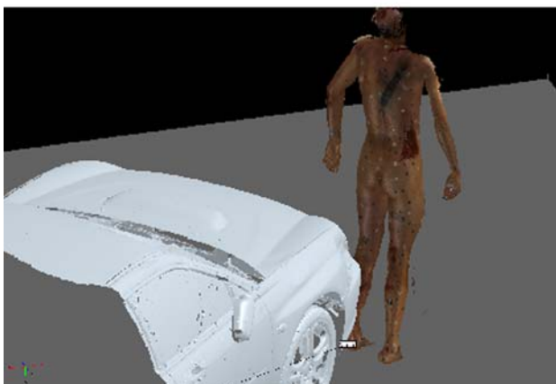
FIG. 15—Case 2: Combined geo-metric 3D surface data sets of the vehicle and the body back in different views.
