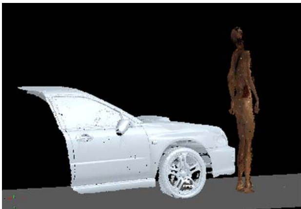
FIG. 14—Case 2: Scanned 3D surface of the car involved in this accident. Note the classical damages in the front parts, the front window and the right rear view mirror.
